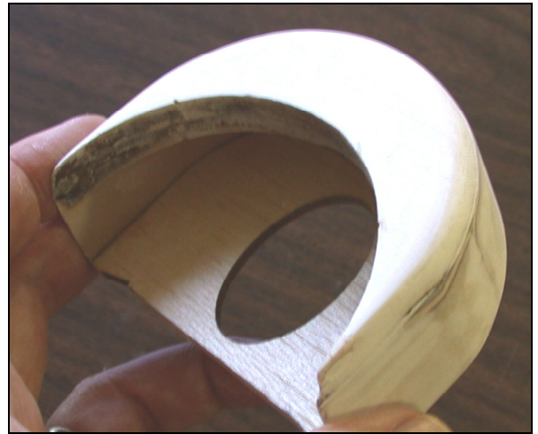
Built up cowl construction
