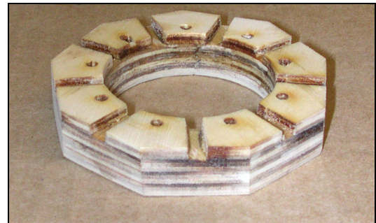
Slots for Cylinder Location Dowels
