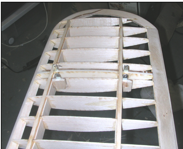
Top Wing Construction Detail
